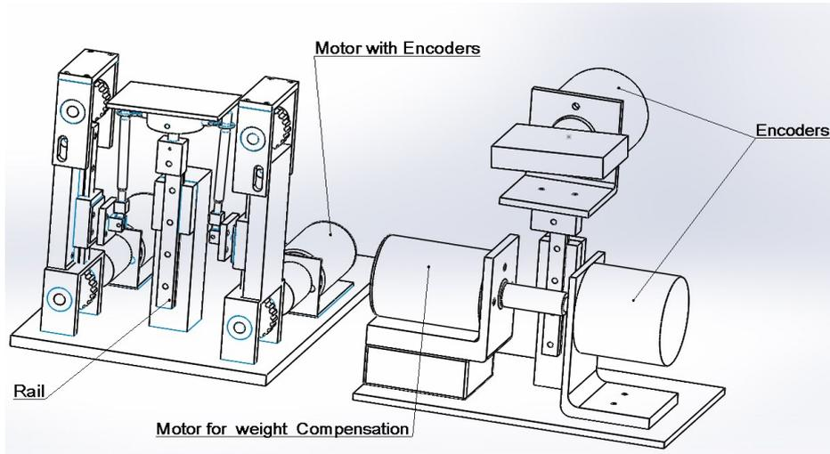
**Figure 2.** Hardware schematics: (left) haptic interface, (right) input device
