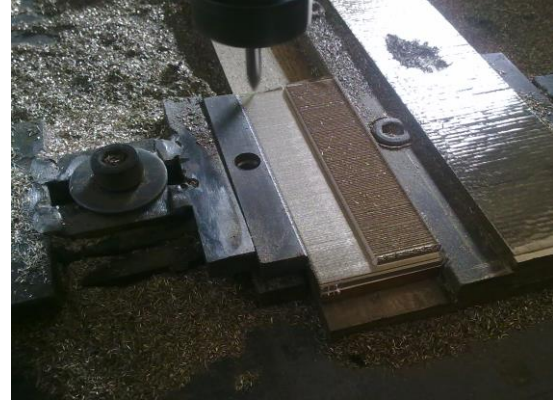
Figure 6. Mold with CNC pantograph machine
