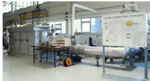
**Figure 1.** Combustion furnace test unit
