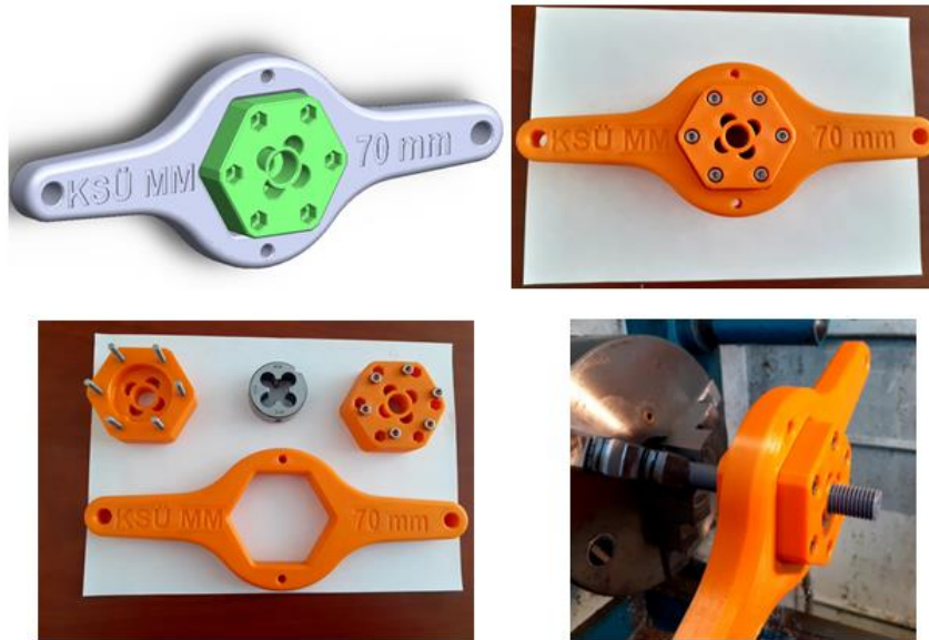
Figure 3. Design and produced novel threading tool
