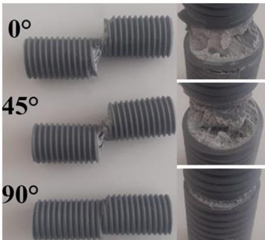
Figure 10. Shear test samples fracture surfaces
