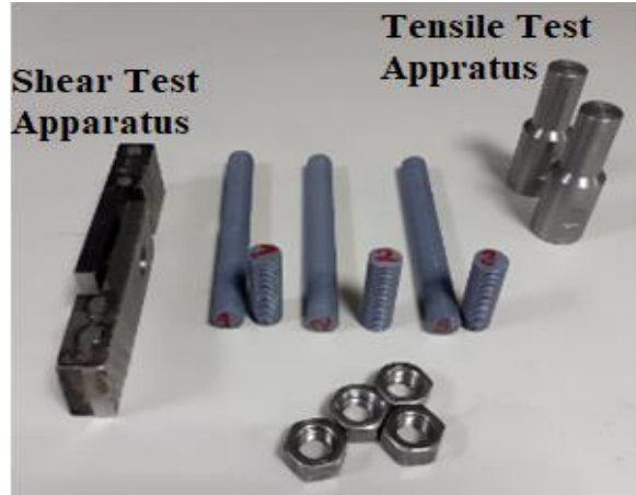
Figure 4. Produced test apparatus and test samples
