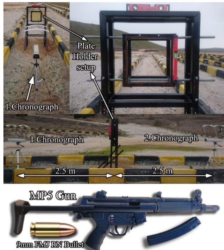
Figure 3. Testing with MP5 gun 9 mm FMJ bullet at the shooting range
