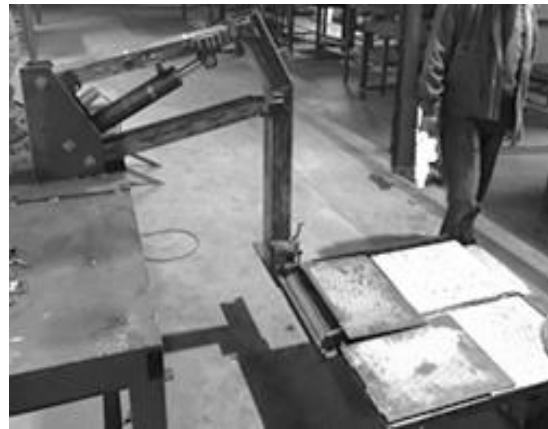
Figure 1. View of the manufactured lift as unfolded
