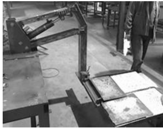
Figure 1. View of the manufactured lift as unfolded
