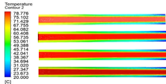
Figure 8. The temperature contours of the RT60 material for different inlet temperatures (From top to bottom, T_{hot,in}=40, 60, 70, 80^\circ\text{C} )
