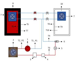
Figure 8. Flow chart of cooling system test unit
