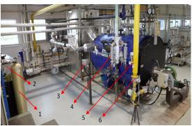
Figure 3. Steam boiler test unit (left side view)
