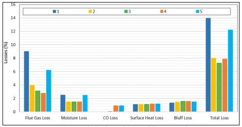
Figure 12. Steam boiler losses in the 5 different experiments
