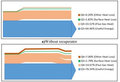
**b)** With recuperator **Figure 10.** Sankey Chart of combustion furnace energy output
