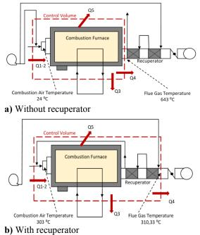
Figure 2. Flow chart of combustion furnace test unit
