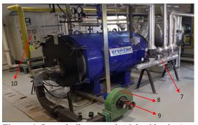
Figure 4. Steam boiler test unit (right side view)
