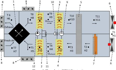
Figure 6. Flow chart of HVAC test unit
