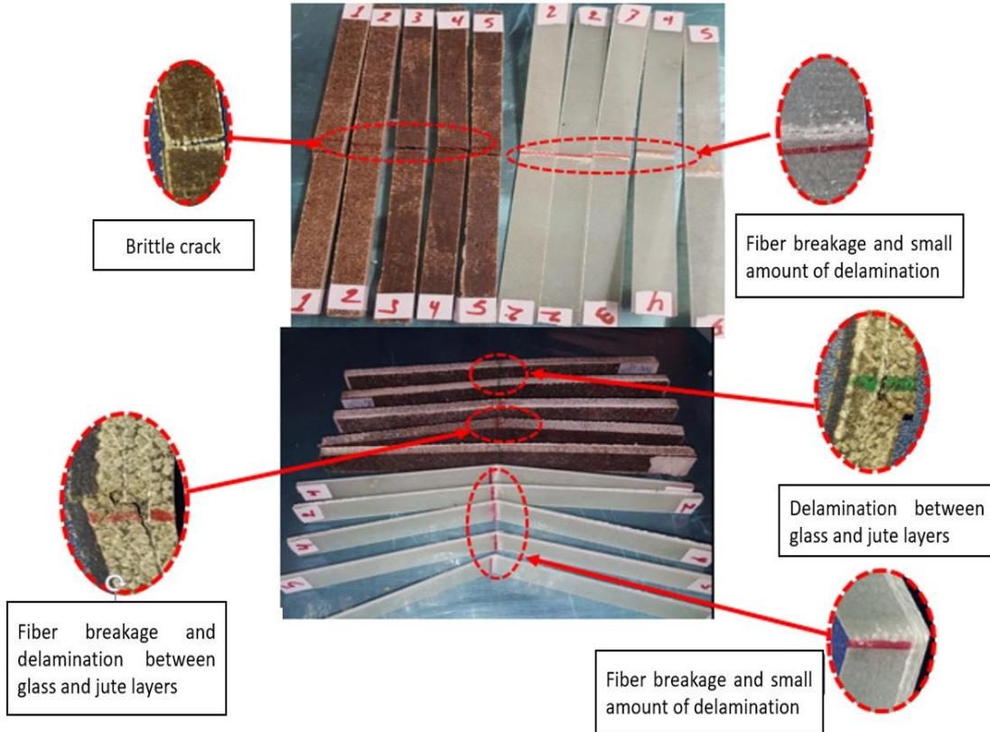
Figure 7. Flexural specimens after the three-point bending test
