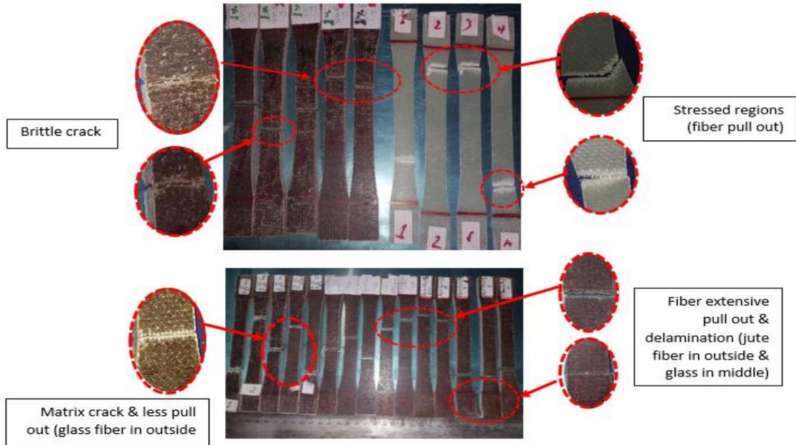
Figure 4. Failure of specimens after tensile test
