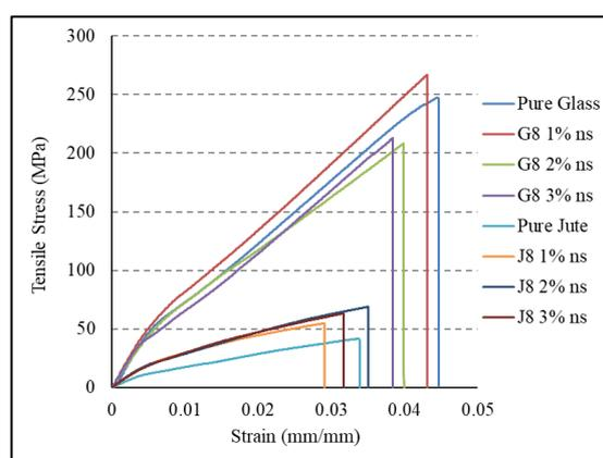
Figure 1. Tensile stress-strain curves of the jute/glass fiber epoxy composite.
