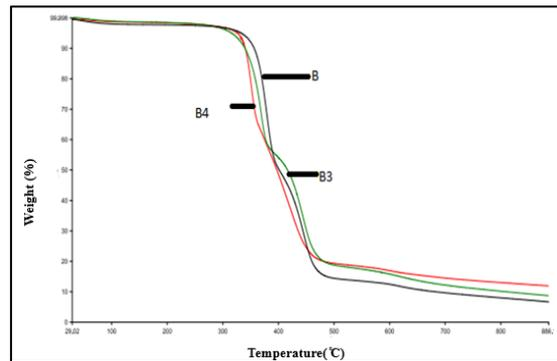
**Figure 11.** TGA arches of 50% CO/50% PES blended fabric (coating method) a-untreated [B] b-150g.licorice root extract [B3] c- 150g. commercial flammable chemical [B4]
