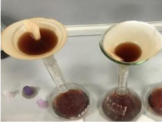
**Figure 2.** Filtration of isopropyl alcohol-licorice root solutions with filter paper
