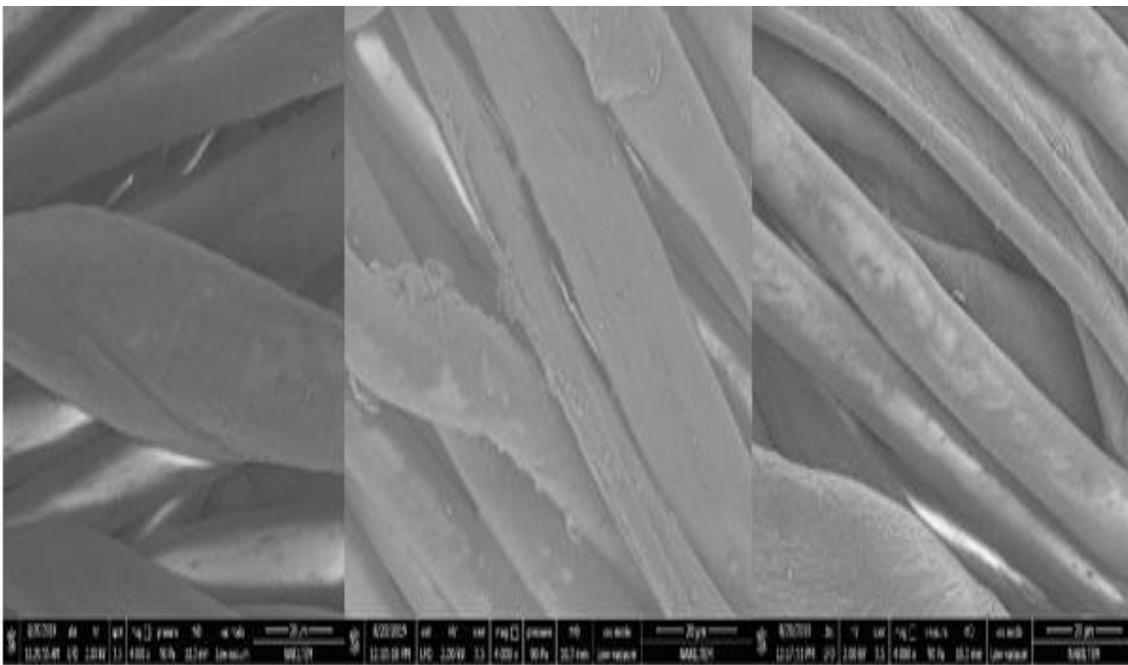
**Figure 7.** SEM images of uncoated Cotton/Polyester blend (a), coated with 150 g licorice root (c), coated with commercial flammable chemical (d)
