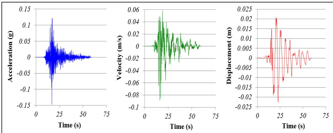
Figure 2. The accelerogram of the Samos-Izmir earthquake [18]
