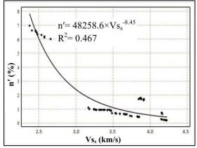
Figure 13. Graph of the relationship between (n') and Vs<sub>s</sub>
