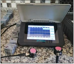
Figure 2. Ultrasonic waves tester
