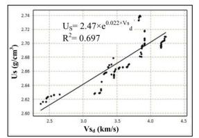
**Figure 5.** Graph of relationship between  $U_s$  and  $V_{S_d}$
