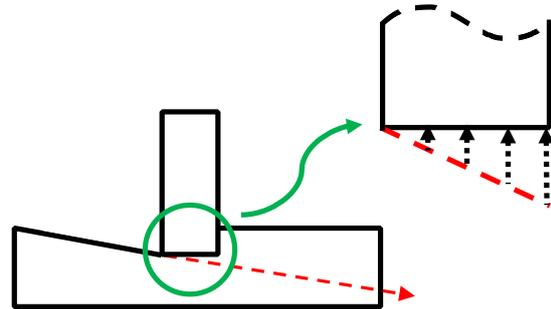
Figure 4. Illustration of cutting forces in VDM [9]
