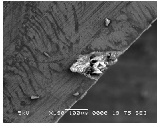
**Figure 1.** Notch wear initiation and propagation [6]
