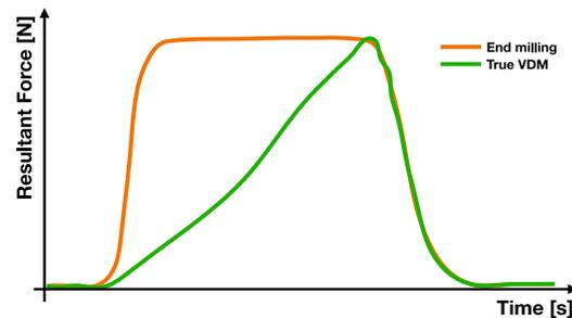
**Figure 6.** Illustration of resultant force development during end milling and true-VDM
