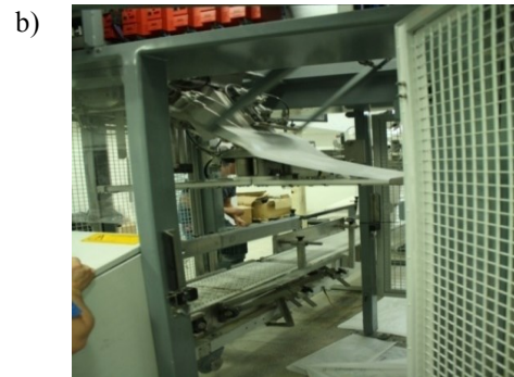
Figure 1. a) Bag placing process in the current packaging plant. b) Bag placing process in the fully automated system
