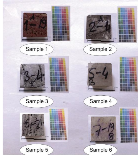
Figure 2. Images of the 30 th cycle after the freeze-thaw test
