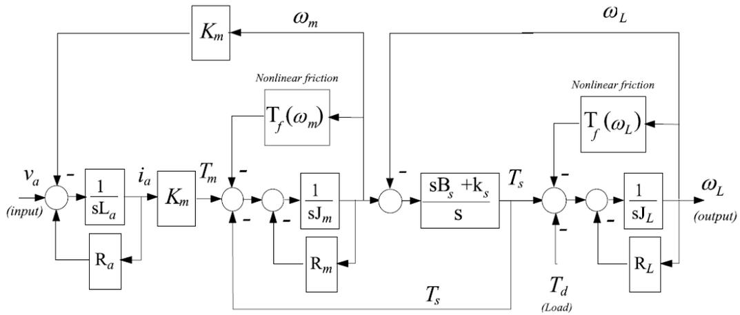
Figure 13. Block diagram of the electromechanical system
