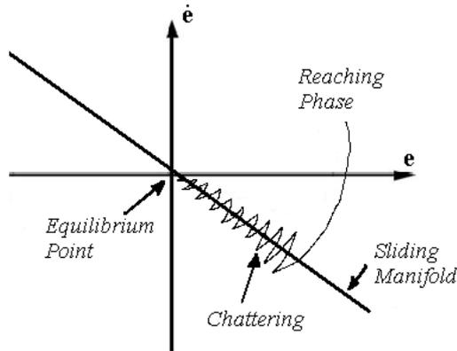
**Figure 1.** Graphical representation of sliding-mode control
