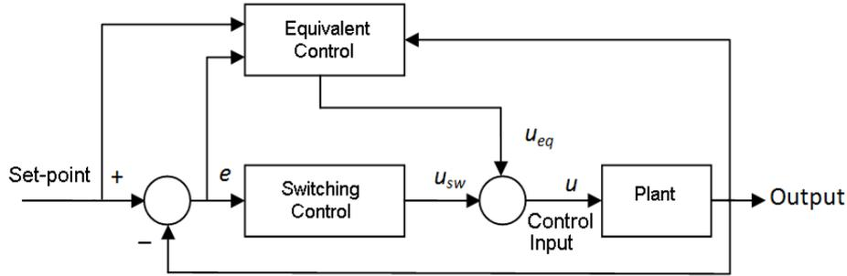
Figure 2. Conventional sliding-mode control for a plant
