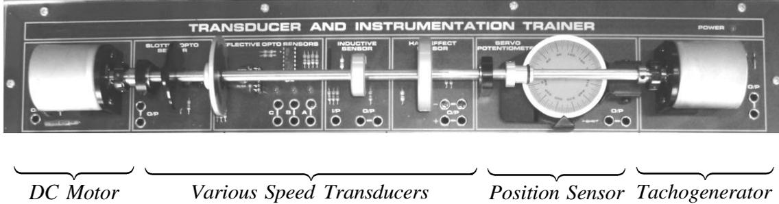
**Figure 3.** A view of the electromechanical system
